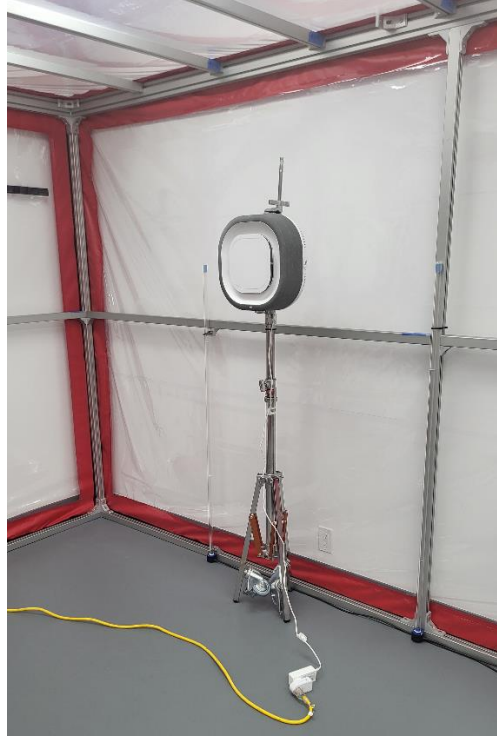
Figure 4. Device mounted 5ft off the floor on a stand located in the center of the 10ft wall.
