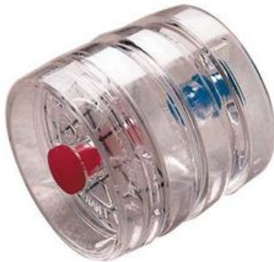
Figure 2: Sensidyne 37mm directionnel air flow sample cassette.
